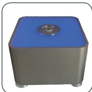
ColorCube benchtop system with a d/8° geometry
